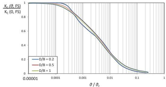
**Figure 10.** Dimensionless chart of the reduction in the coupled swaying-rocking stiffness with increasing rotation, for zero displacement and full contact conditions.
