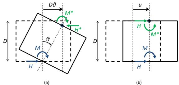
**Figure 2.** Sub-cases of Figure 1: (a) imposed rotation at the base with constrained displacement and (b) imposed horizontal displacement with constrained rotation.
