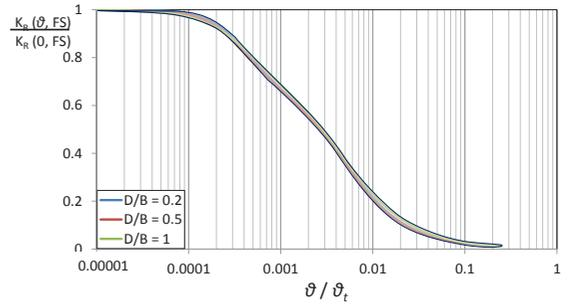
**Figure 9.** Dimensionless chart of the reduction in the rocking stiffness with increasing rotation, for zero displacement and full contact conditions.
